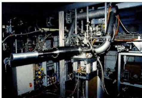
Fig. 2. The horizontal dilution refrigerator used for the Gerasimov-Drell-Hearn experiment at the Mainz microtron, MAMI. The target material, with a volume of about 6\text{ cm}^3 , is located within the front end of the cryostat.
